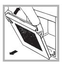
3. Grip the door on the two external sides and close it approximately half way. Pull the door towards you lifting it out of its seat (*see diagram*). To replace the door, reverse this sequence.
